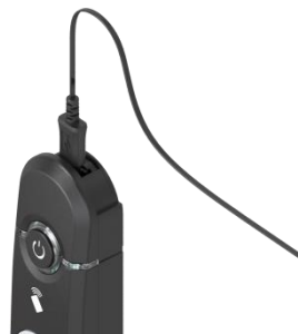
Fig. 7: Remove USB cover, connect to laptop or mobile phone charger for powering up in case of battery failure
