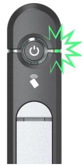
Fig. 4: With valid RFID card, right LED starts blinking and handle opens. Red LED indicates invalid card
