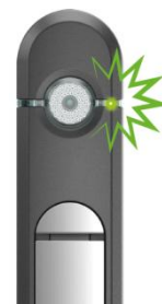
Fig. 4: With valid RFID card, right LED starts blinking and handle opens. Red LED indicates invalid card
