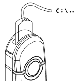
Fig. 6: Emergency opening via USB port; requires special software and USB <-> USB micro adaptor cable
