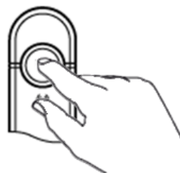
Fig. 5: With right LED blinking, touch sensor field to open the handle
