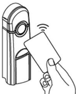
Fig. 4: Show card to reader left LED is lit if valid card type detected. Right LED starts blinking if card is authorized
