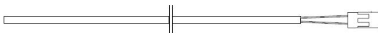
Fig. 2: Connecting cable (part-no. 2807) for Agent E swing handles; overall lengths about 2.0 m
