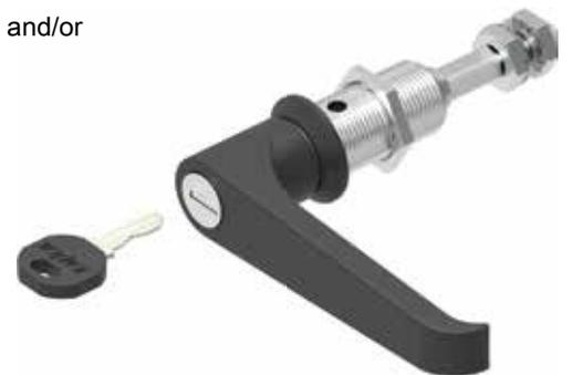
Handle and housing zinc die black powder coated, cylinder zinc die with stainless steel cap and dust cover, nut and screw zinc plated with spring and seal. Each cylinder has one silver steel key with polyamid grip. Key removable in both positions
