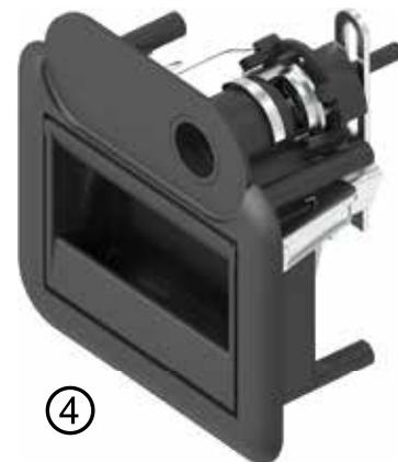
**Exterior handle polyamide GF black; pivot m.s. zinc plated; pivot arm zinc die zinc plated; with spring**
