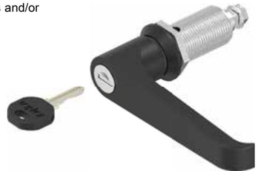
Handle and housing zinc die, black powder coated, cylinder zinc die, with stainless steel cap and shutter, nut and screw zinc plated m.s. with spring and seal. Each cylinder has one silver steel key with polyamid grip. Key removable in both positions
