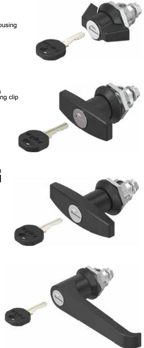
Handle polyamide GF black / zinc die, housing polyamide GF black, round cylinder zinc die with stainless steel cap and dust cap, screw m.s. zinc plated, with seal. Each cylinder has one silver steel key with polyamid grip. Key removable in both positions
