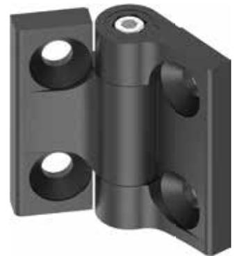
**180° Screw-on torque hinge zinc-die black powder-coated for countersunk screw M8; friction cone polyacetal POM; screw and nut m.s. zinc-plated**
