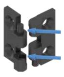
The two identical hinge halves are plugged into each other in the 270° position.
